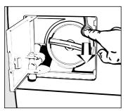
Pull the ring of the door mechanism downwards, and the door will open.
